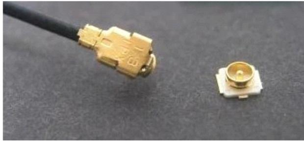
Figure 22 USR-WIFI232-T 外置天线接头示意
