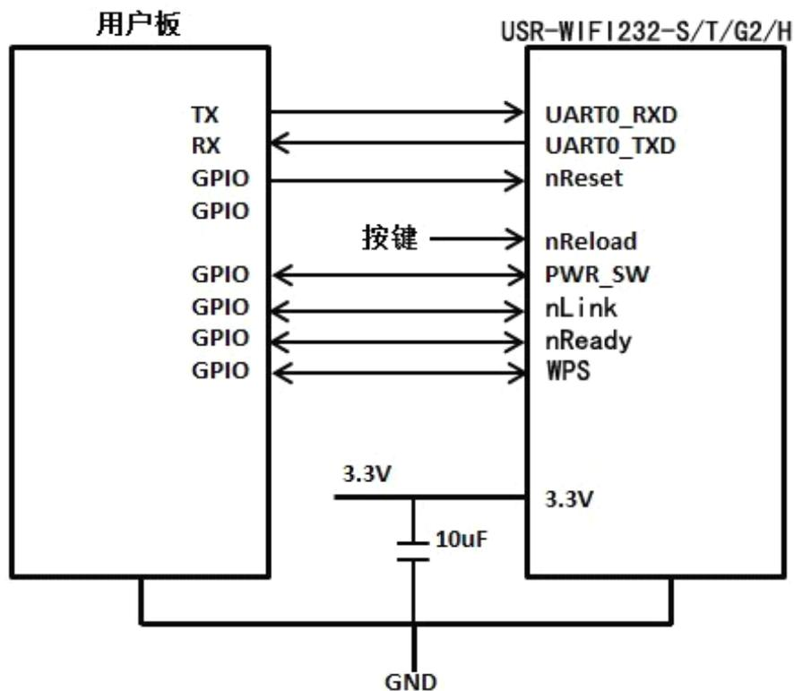
Figure 25 USR-WIFI232-S/T/G2 UART 应用硬件连接
