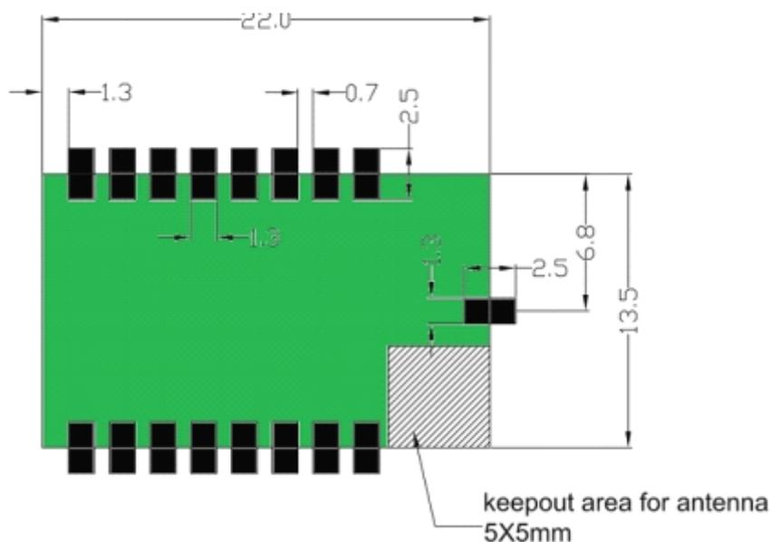
Figure 17 USR-WIFI232-S PCB 元件尺寸
