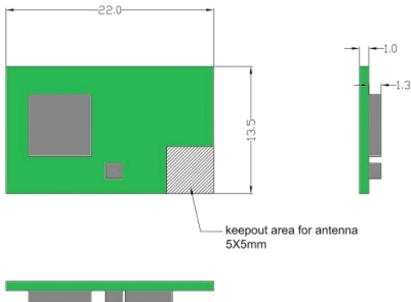
Figure 16 USR-WIFI232-S 机械尺寸
