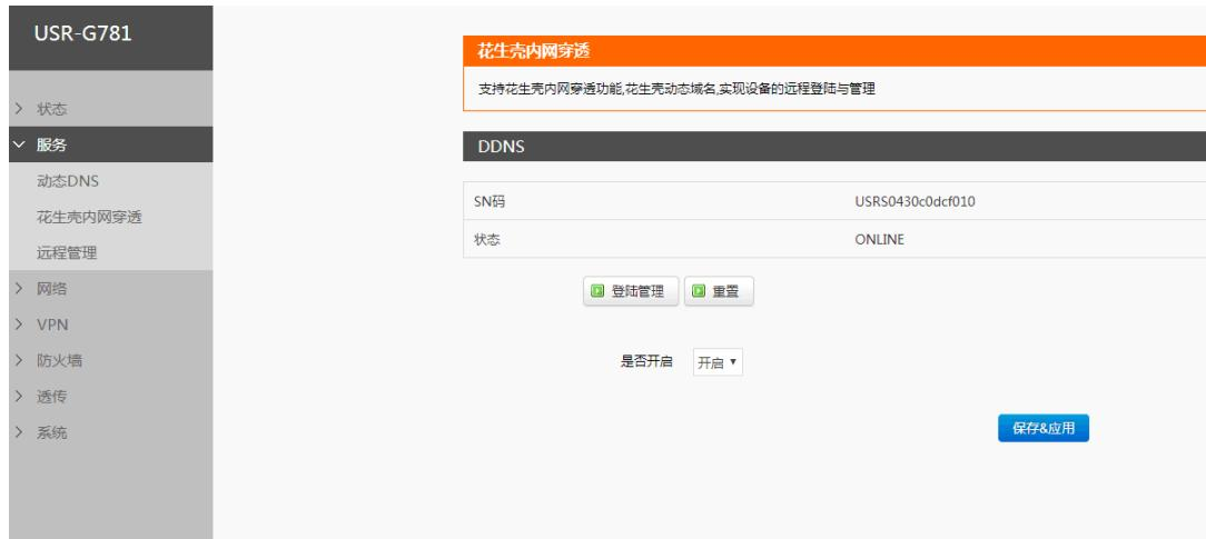
The screenshot shows the花生壳内网穿透 configuration after a restart. The status is now ONLINE, and the SN code is USRS0430c0dcf010. The checkbox for '是否开启' is now unchecked. A blue '保存&应用' (Save & Apply) button is at the bottom right.
