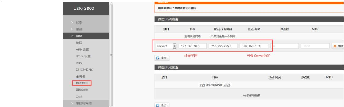
The screenshot shows the 'USR-G800' web interface under the 'Network' section. In the 'Static Routing' tab, there is a table for 'Static IPv4 routes'. One row is highlighted with a red box, showing 'server1' as the interface, '192.168.20.0' as the destination, '255.255.255.0' as the subnet mask, and '192.168.0.10' as the gateway.
