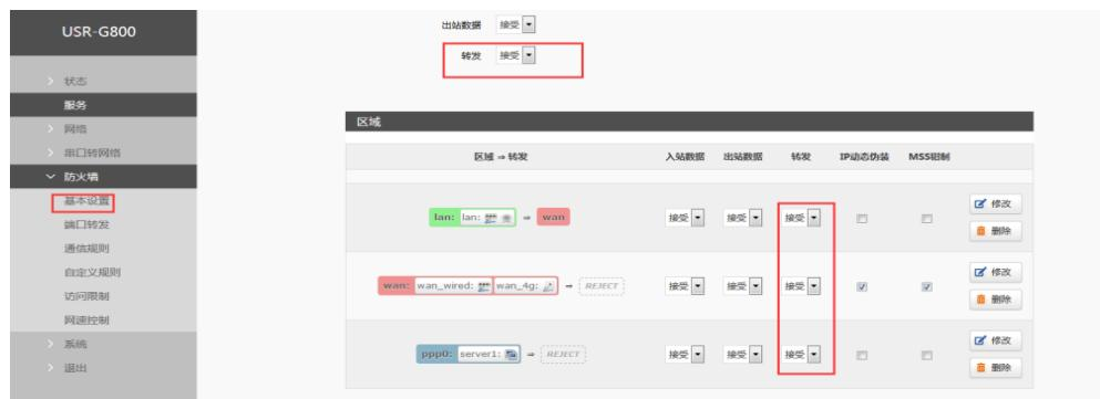
The screenshot shows the 'USR-G800' web interface under the 'Firewall' section. In the 'Basic Settings' tab, there is a table for 'Zone' rules. One rule is highlighted with a red box, showing 'wan' as the source interface, 'wan' as the destination interface, and 'REJECT' as the action.
