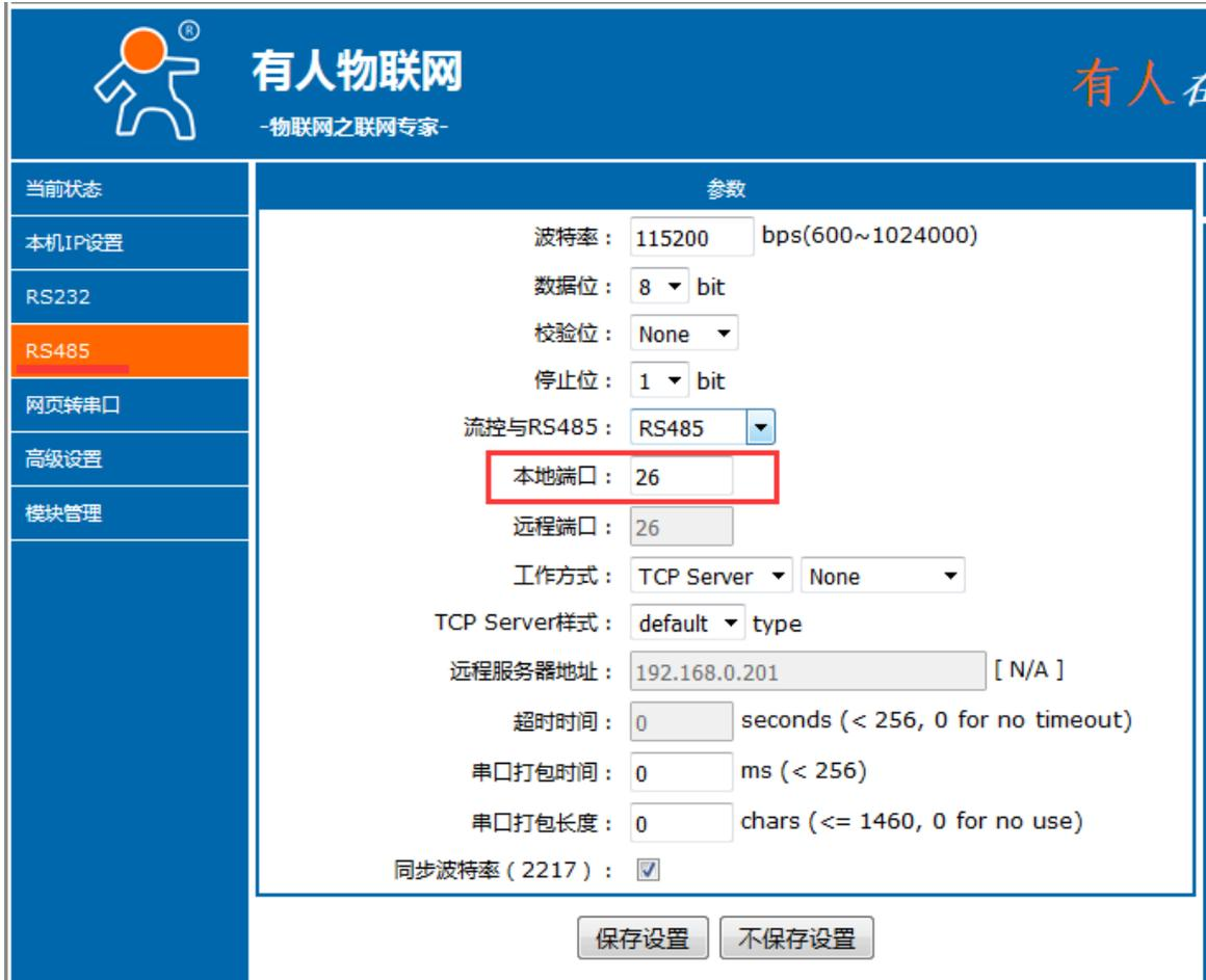
The screenshot shows the configuration web interface for the USR-TCP232-M4 device. The interface is in Chinese and features a blue header with the '有人物联网' (Youren IoT) logo and tagline '物联网之联网专家'. A left sidebar contains navigation options: '当前状态', '本机IP设置', 'RS232', 'RS485' (highlighted in orange), '网页转串口', '高级设置', and '模块管理'. The main content area is titled '参数' (Parameters) and lists various settings for RS485:
