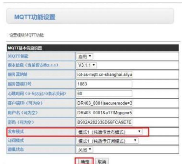
The screenshot shows the 'MQTT功能设置' (MQTT Function Setting) page. It has a sub-header '设置模块MQTT功能' (Set MQTT Function Module). Below is a table for 'MQTT基本信息设置' (MQTT Basic Information Setting) with the following fields:
